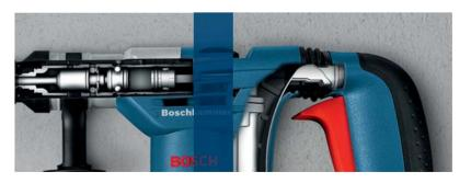
Example: GBH 4-32 DFR Professional. 1st stage: The air buffer, which is larger than in conventional hammer mechanisms, reduces the air pressure in the hammer mechanism. This counteracts the oscillations like a spring and dampens the vibrations where they originate: in the hammer mechanism. 2nd stage: The main handle is decoupled from the machine by means of a leaf spring and two swivel joints. The vibrations already reduced by the first stage are absorbed further.
